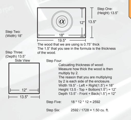
Calculating a speaker enclosure volume with a port is a seven step process. The First six steps are the same as the sealed enclosure. The only difference is calculating the port displacement.
